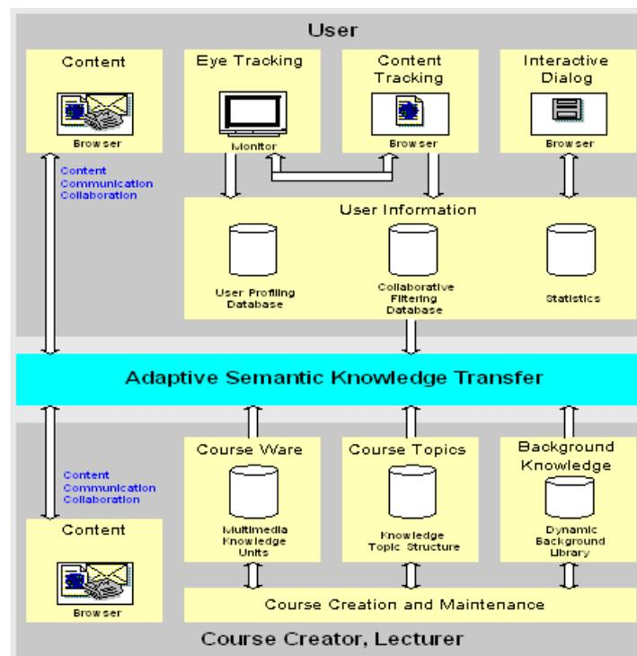
**Figure 2.** The architecture of the AdeLE framework.
